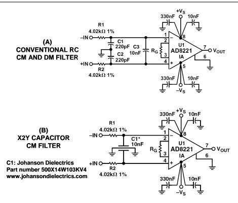
Figure 5: Conventional RC and X2Y CM Filters
