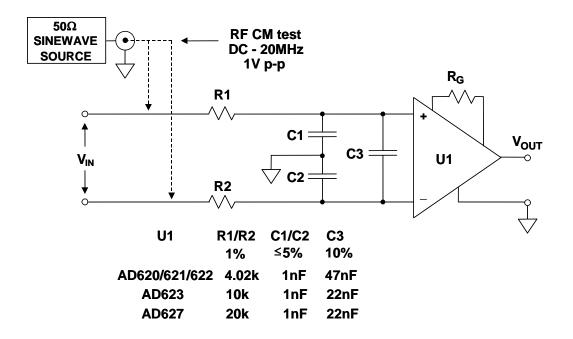
Figure 2: Flexible Common-Mode and Differential-Mode RC EMI/RFI Filters are useful with the <u>AD620</u> Series, the <u>AD623</u>, <u>AD627</u>, and other In-Amps
