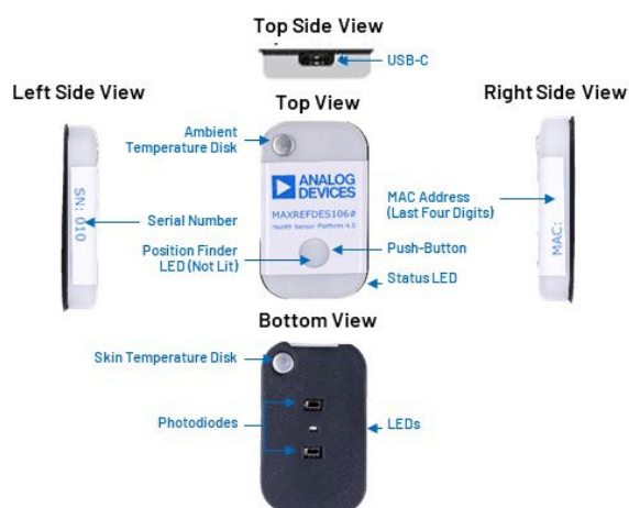
Figure 2. A MAXREFDES106# annotated hardware diagram (32 mm × 52 mm).
