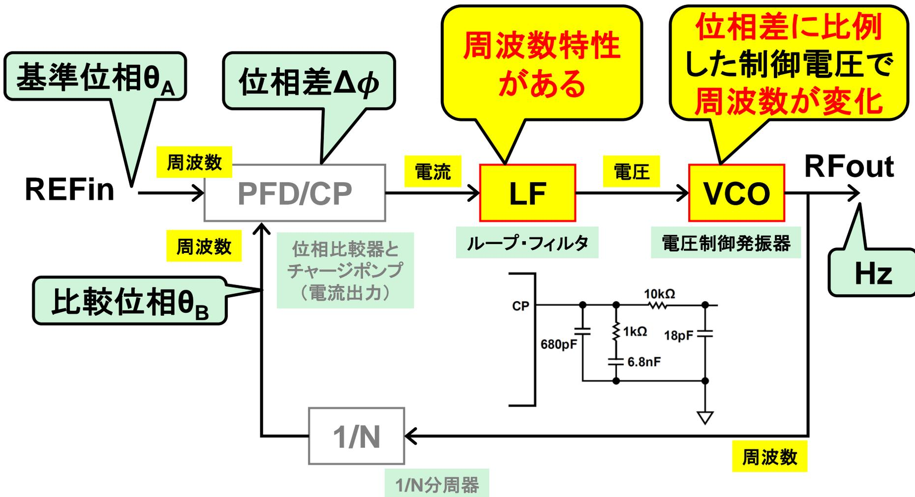
$$\Delta\phi[\text{rad}] = \theta_A [\text{rad}] - \theta_B [\text{rad}] \quad (\text{周波数の時間積分が位相})$$
