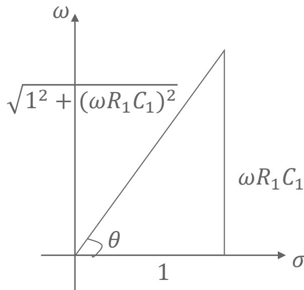
$$\frac{G(j\omega)}{|G(j\omega)|} = \frac{\frac{1}{R_1 C_1 s + 1}}{\frac{1}{\sqrt{1 + (\omega R_1 C_1)^2}}} = \frac{1}{\sqrt{1 + (\omega R_1 C_1)^2} + j \frac{\omega R_1 C_1}{\sqrt{1 + (\omega R_1 C_1)^2}}} = e^{j\alpha}$$
