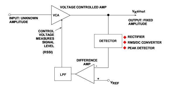
Figure 2: A Typical Automatic Gain Control (AGC) System
