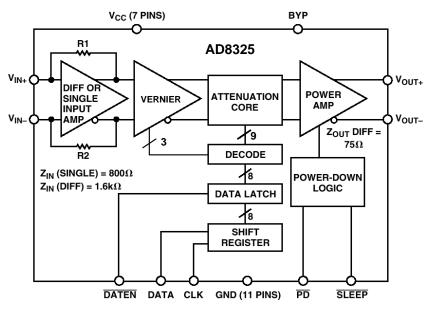
Figure 8: AD8325 CATV Digitally Controlled Variable Gain Amplifier
