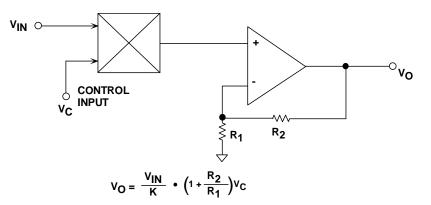
Figure 3: Using a Multiplier as a Voltage-Controlled Variable Gain Amplifier
