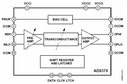
Figure 9: AD8370 750MHz Digitally Controlled VGA
