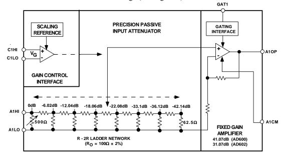
Figure 4: X-Amp Block Diagram
