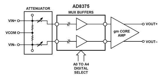
Figure 10: AD8375 630MHz Low Distortion Digitally Controlled VGA
