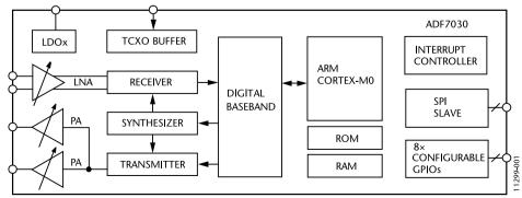
Figure 1.2 ADF7030 block diagram [3].
