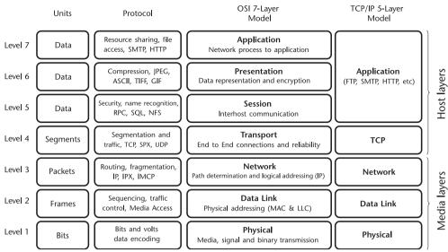
Figure 1.4 Seven-layer OSI model compared to five-layer TCP/IP model.
