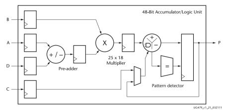
Figure 1.9 Basic DSP48E1 slice functionality [5].
