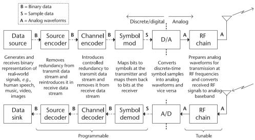
**Figure 1.3** An illustration describing some of the important components that constitute a modern digital communications system. Note that for a SDR-based implementation, those components indicated as programmable can be realized in either programmable logic or software.
