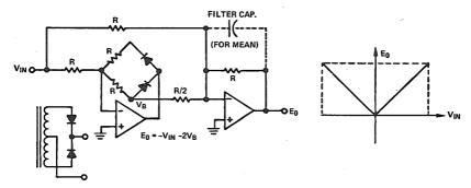
Applications in precision instrumentation include AC measurements, function fitting, inputs to single-quadrant devices (squarers or vector sums), triangular-wave frequency doubling, and error measurements.
