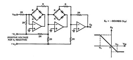
Precision bounds are useful in setting, or simulating, limits to voltage or current (or its rate-of-change), in establishing thresholds of ranges of operation in piecewise-linear function fitting, and (preceded by comparators) in establishing precise voltage staircase functions (i.e., quanta).
