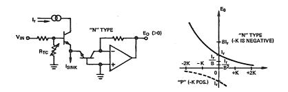
Antilog devices use the same circuitry as log devices; the distinction lies in the way they are connected. The log transistor and its temperature-compensating circuitry develop a current that is proportional to the antilogarithm of the applied voltage. If the applied voltage is the input signal, the op amp, with a feedback resistor, develops an exponential output voltage; if the applied voltage is
