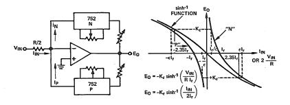
If the antilog elements are connected in the input path, the inverse function, i.e., the hyperbolic sine, is generated.
