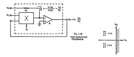
One should not expect an analog divider to be capable of division by zero, or by bipolar numbers. (With switching, 4-quadrant division is feasible — away from zero.) Generally, the problem can be restated to eliminate such anomalous operations. A divider can, of course, compute reciprocals if the numerator is held fixed at an appropriate constant value.
