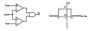
Jump functions are useful in sensing polarity, in precisely locating thresholds, and for all of the applications mentioned under Comparators. The window function can be used for precise quantization, for grading and sorting, and for pulse-width modulation. A comparator and a window can be used in conjunction to initiate a function that depends on the sign and quantized magnitude of a voltage.
