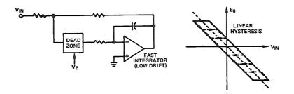
Besides two-level hysteresis, there is also "linear" hysteresis, best-known to electrical engineers in the form of magnetic "remanence," and to mechanical engineers as "backlash" in gear trains. Devices with linear hysteresis follow the input in one direction; when the direction of input is reversed, a dead band must be traversed before the output follows.
