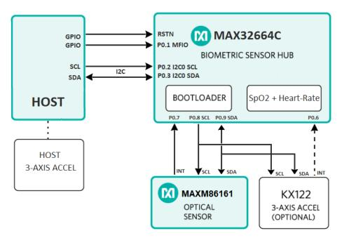
Figure 2. Architecture diagram for health-sensing applications using an I<sup>2</sup>C interface to communicate with the sensor (such as the MAXM86161).
