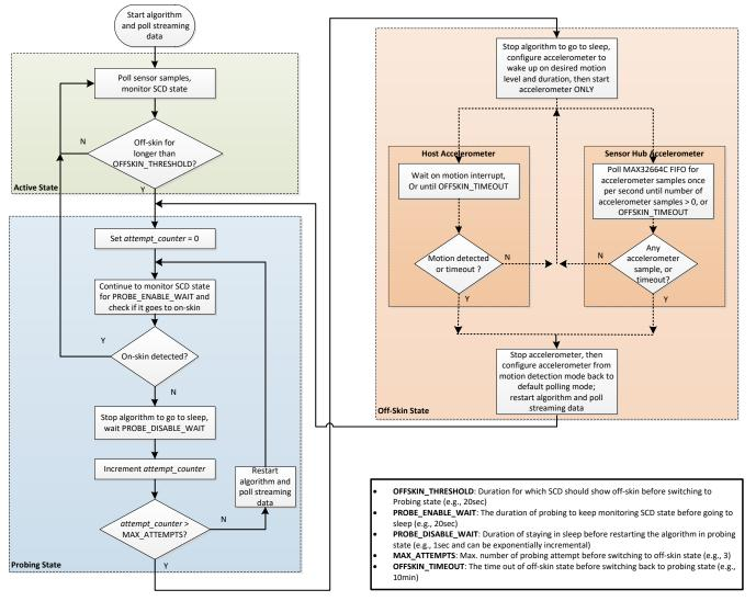
Figure 4. Example of an SCD-enabled, power-saving state machine.
