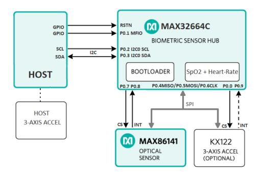
Figure 1. Architecture diagram for health-sensing applications using an SPI interface to communicate with the sensor (such as the MAX86141).
