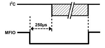
Figure 3. Host interface signaling.
