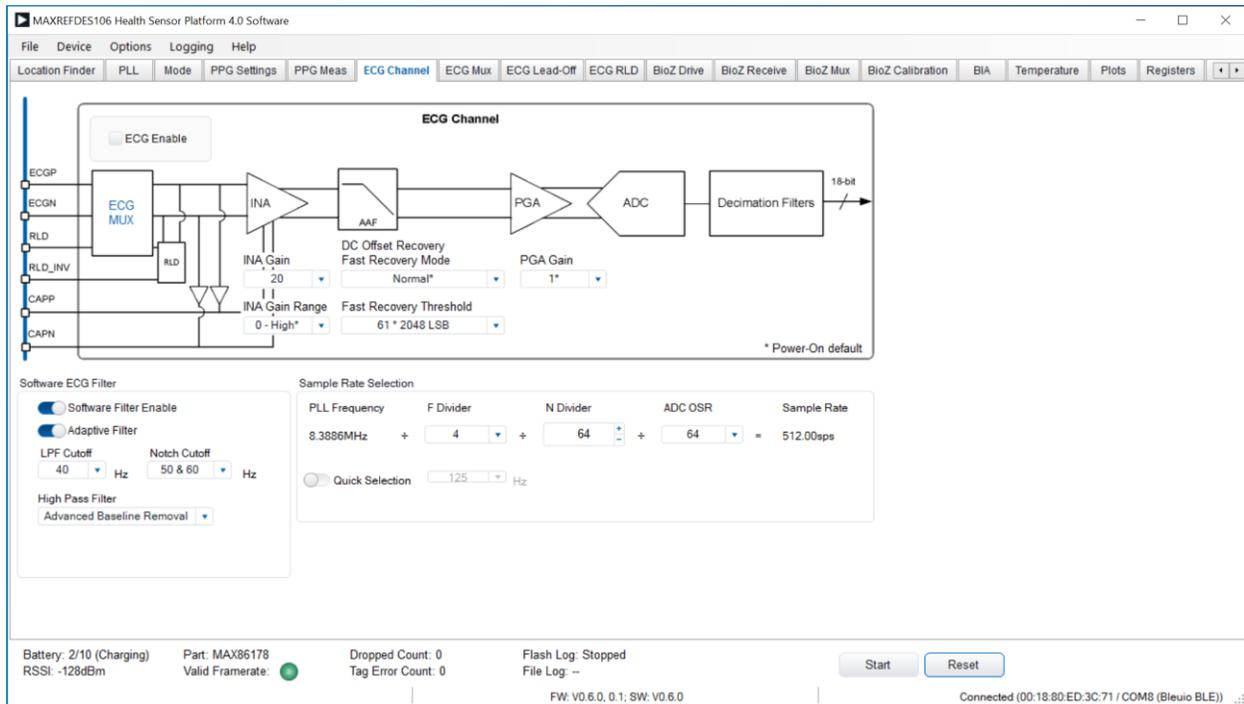
Figure 56. ECG Channel Tab
