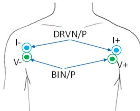
Figure 29. BioZ Electrodes: I- (Blue), I+ (Blue), V- (Green), V+ (Green)
