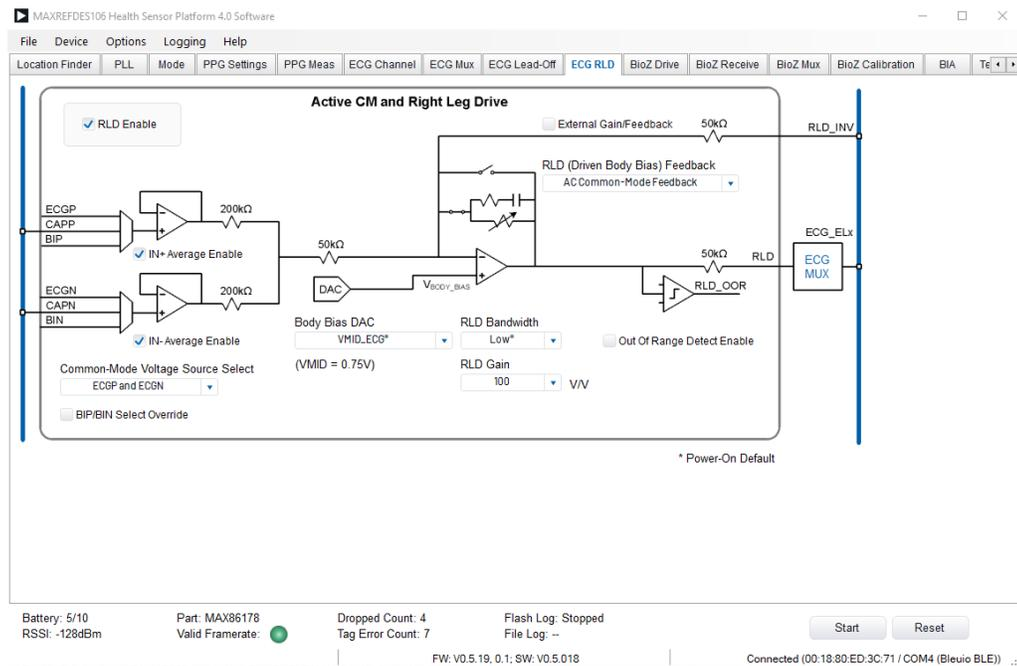
Figure 45. ECG RLD Tab
