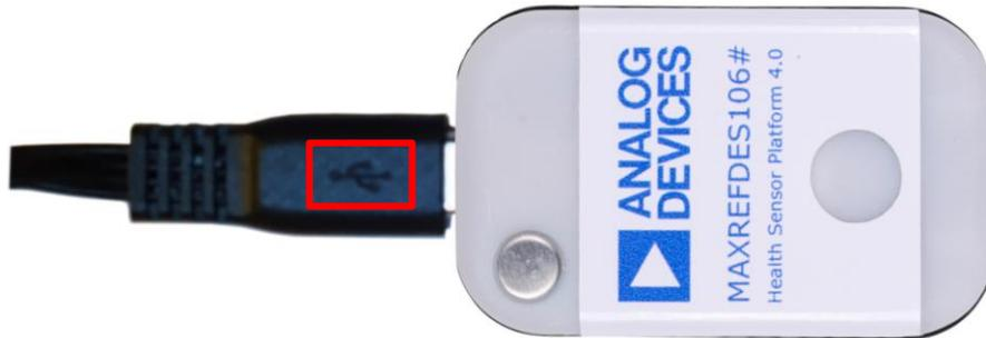
Figure 21. Orientation of the USB-C 7-Lead Electrode to the MAXREFDES106#
