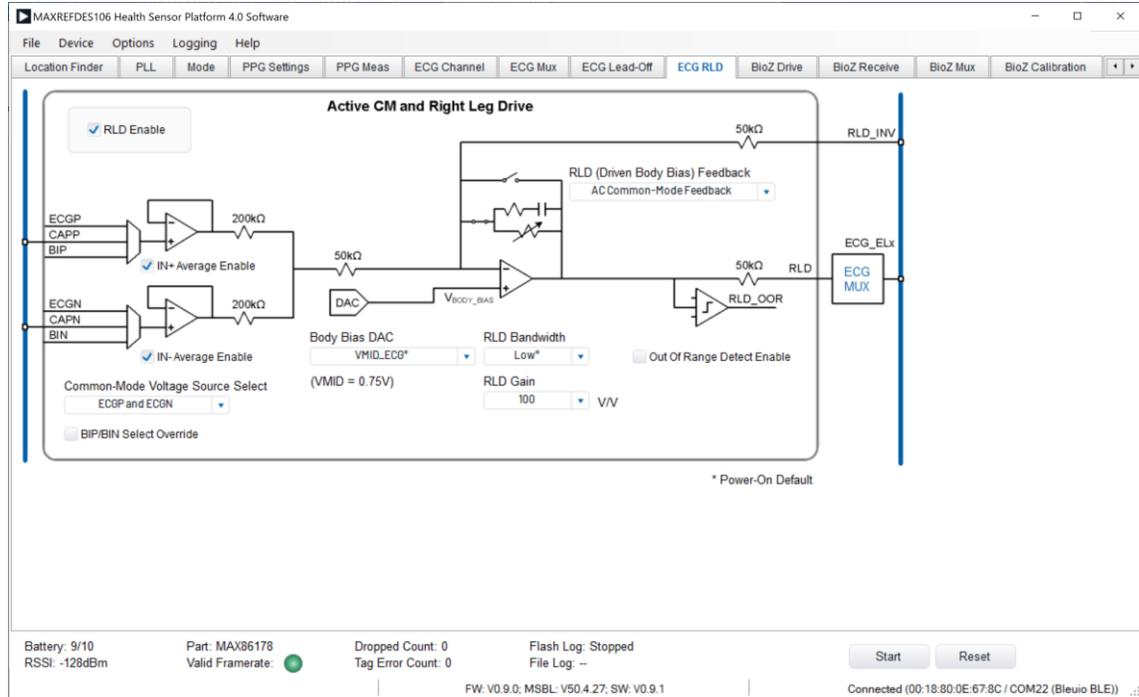
Figure 34. ECG RLD Tab: Use Power-On Default Settings
