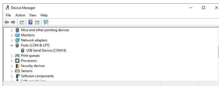
Figure 86. Note the USB Serial Device COM Port Number for the BleuIO Dongle During the First Nine Seconds
