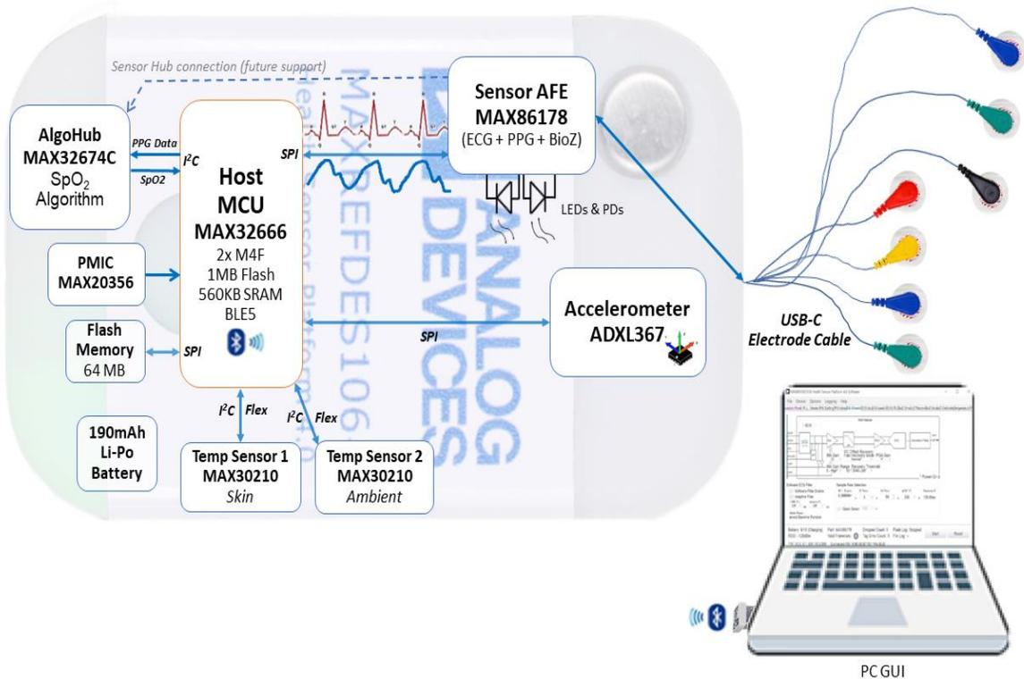
Figure 2. MAXREFDES106# System Diagram
