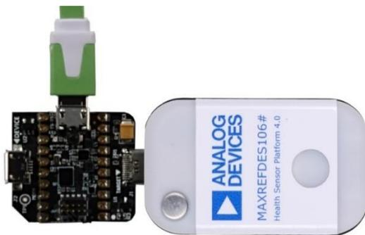
Figure 3. Micro-USB to MAXDAP-TYPE-C to MAXREFDES106#.
