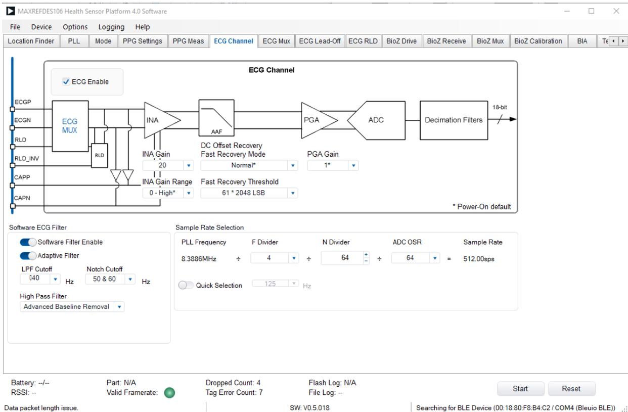
Figure 42. ECG Channel Tab: Use Power-On Default Settings
