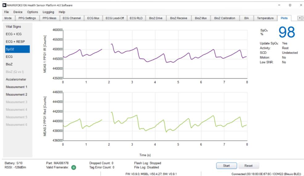
Figure 47. Example SpO<sub>2</sub> Algorithm Output
