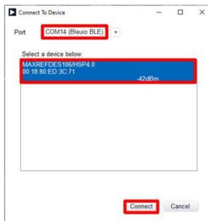
Figure 18. Connect the PC GUI BleuIO to the MAXREFDES106#
