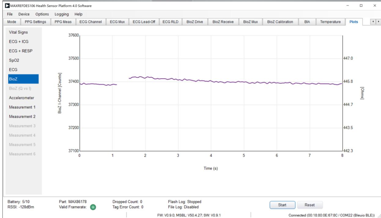
Figure 28. Example BioZ Measurement Output
