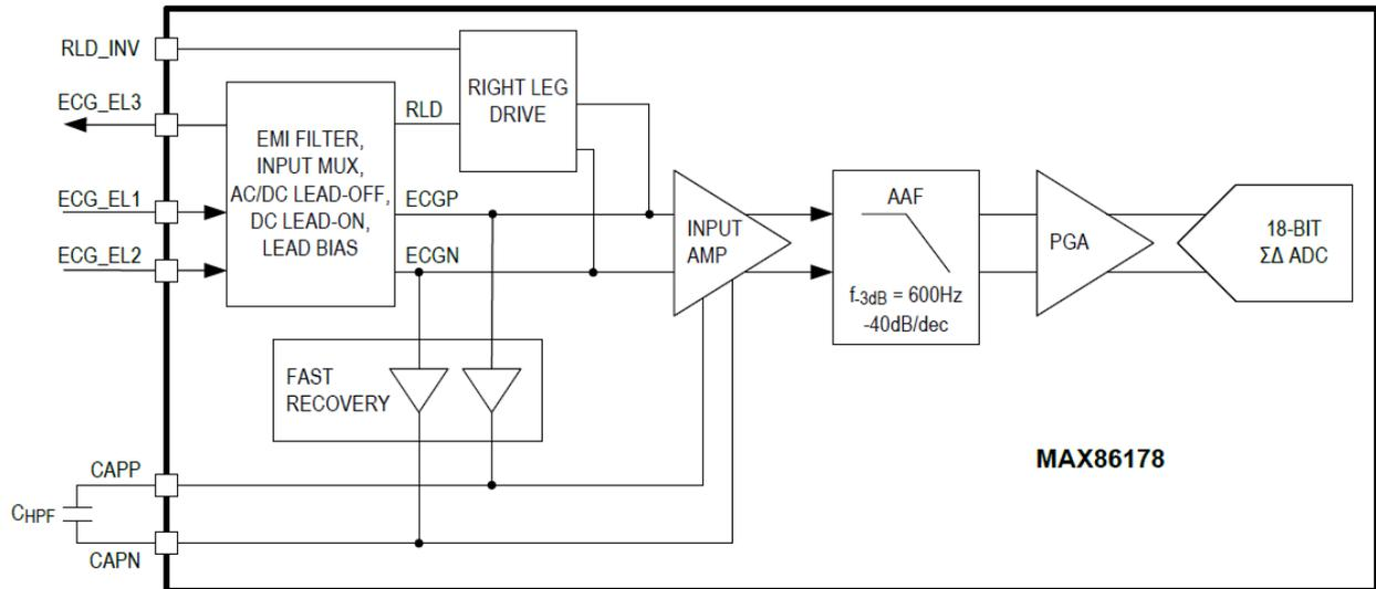
Figure 25. ECG Channel Signal Chain
