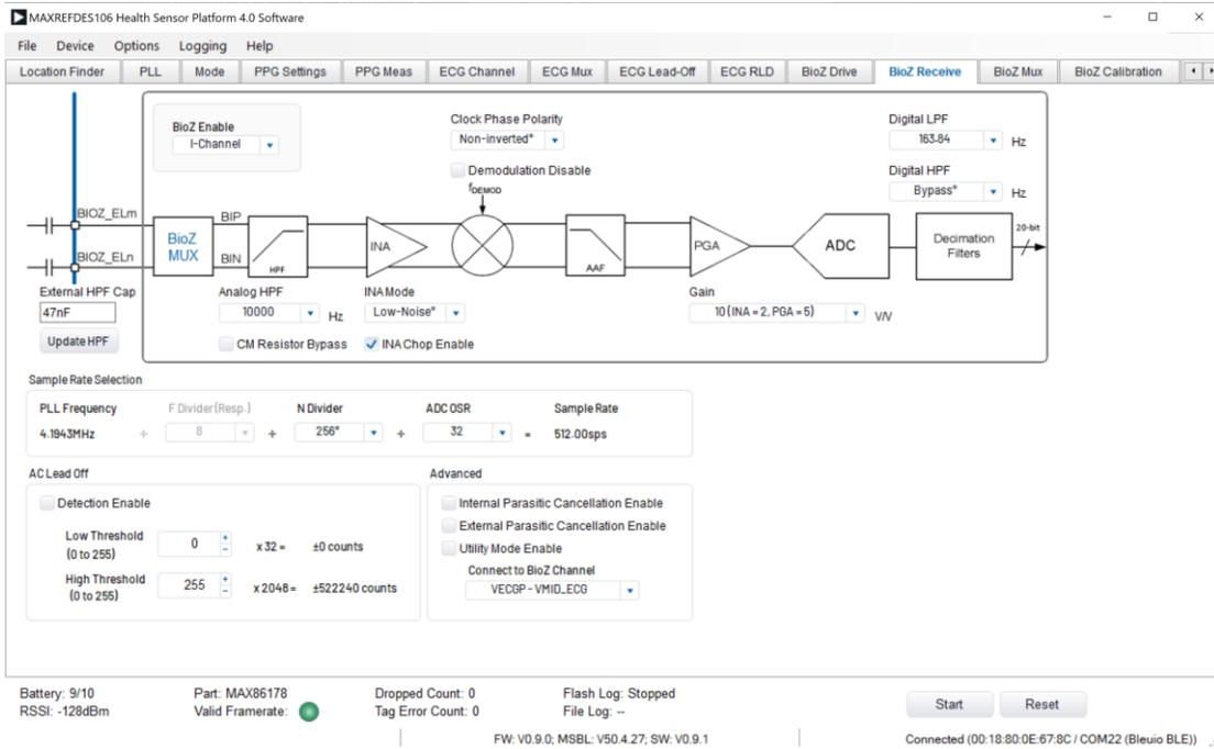
Figure 36. BioZ Receive Tab: Use Power-On Default Settings
