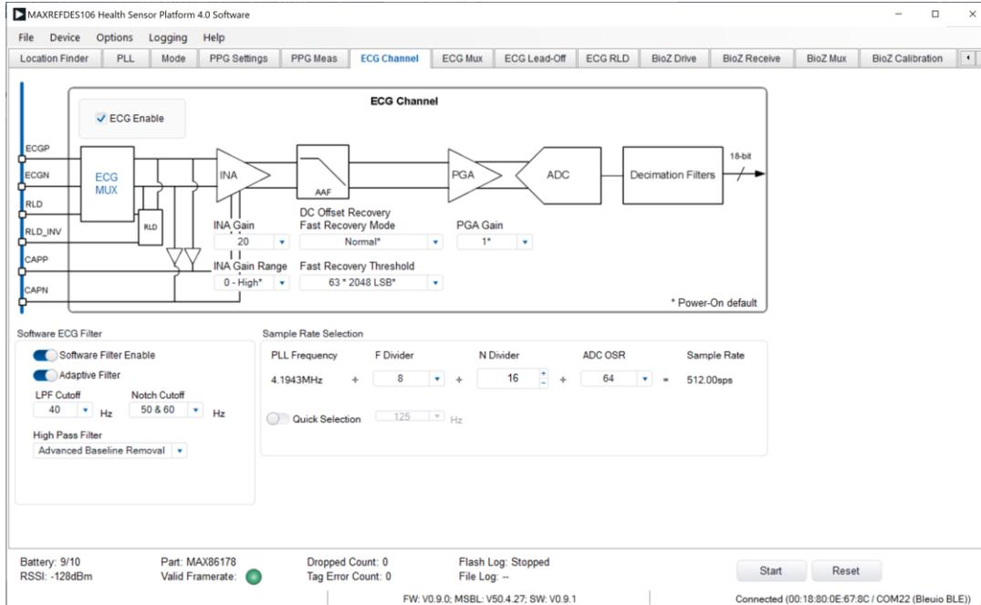
Figure 32. ECG Channel Tab: Use Power-On Default Settings
