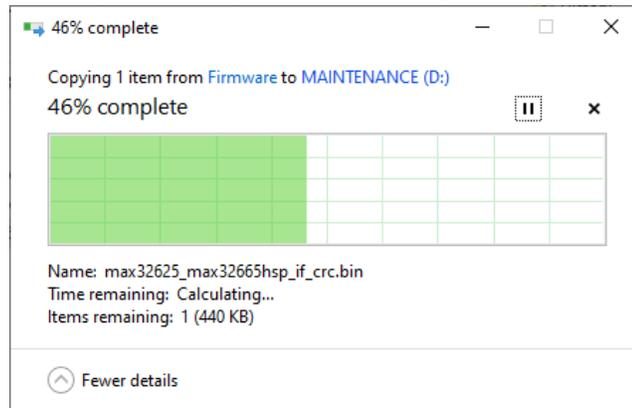
Figure 78. Wait for the Percent Complete Message to Finish and the MAXDAP-TYPE-C LED to Stop Flashing
