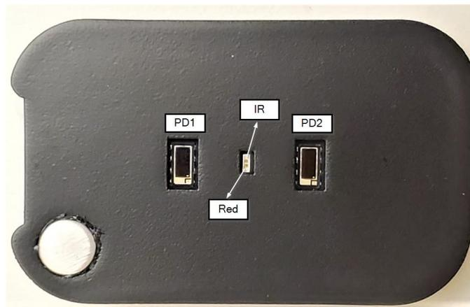
Figure 55. MAXREFDES106# LED and PD Layout, Bottom View
