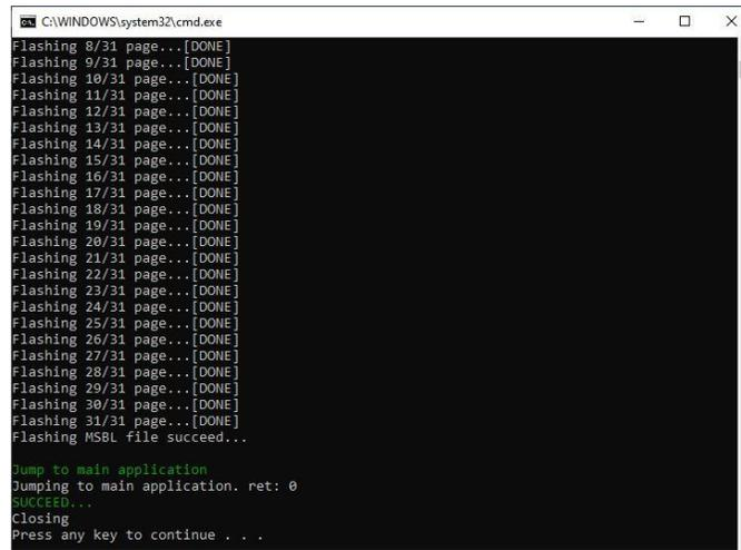
Figure 10. Flashing the .msbl to the MAX32674C
