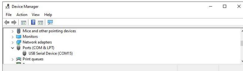
Figure 82. After the BleuIO is Plugged in for at Least 10 Seconds, Note the USB Serial Device COM Port Number for the BleuIO Dongle
