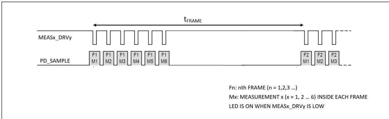
Figure 22. Frame with Six Measurements, M1 to M6
