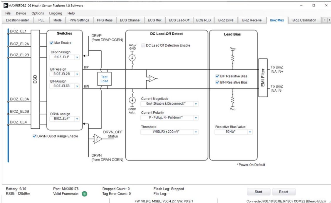
Figure 37. BioZ Mux Tab: Use Power-On Default Settings
