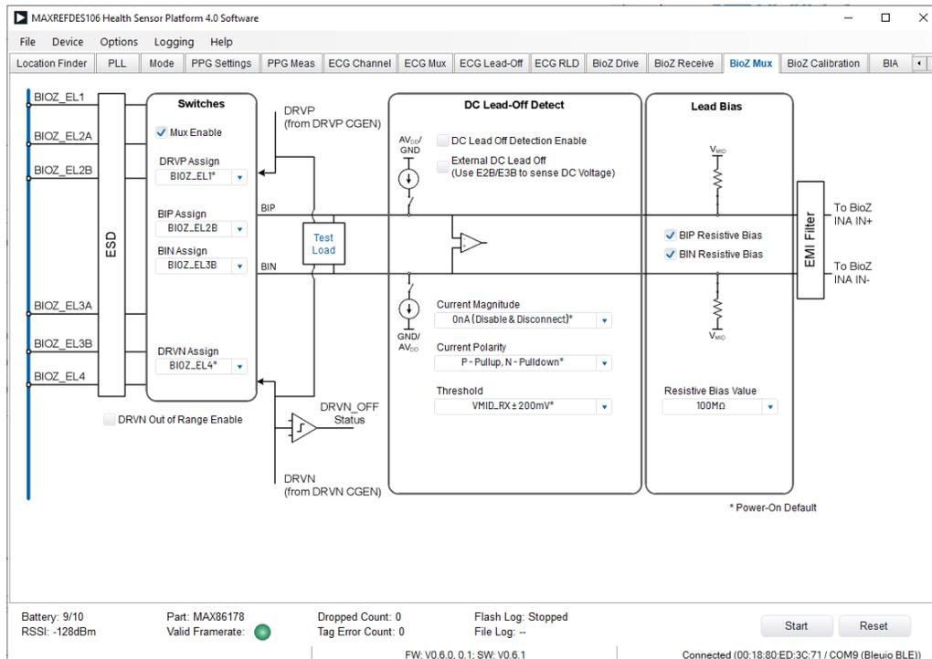
Figure 62. BioZ Mux Tab
