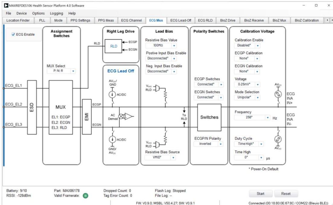
Figure 33. ECG Mux Tab: Use Power-On Default Settings
