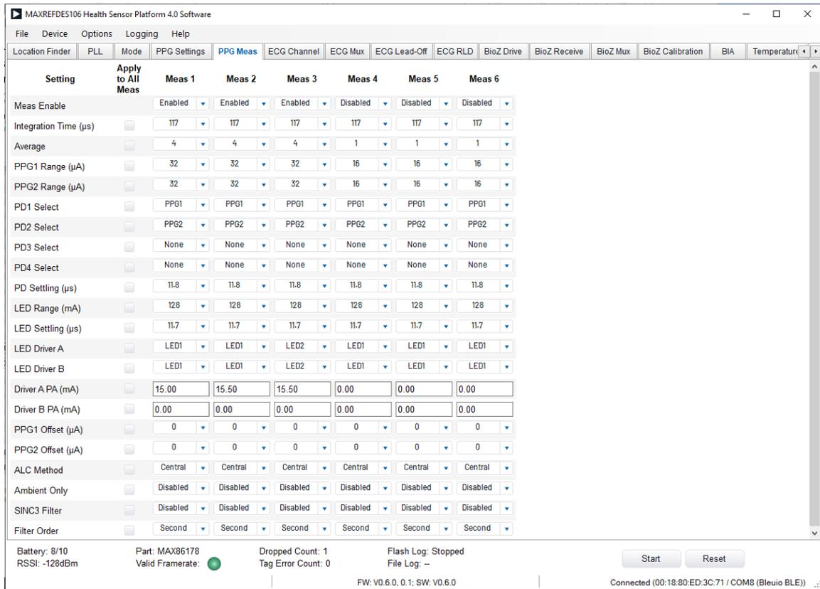
Figure 54. PPG Meas Tab: PPG Measurement Settings Tab
