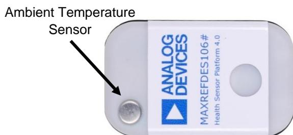
Figure 48. MAXREFDES106# Thermal Contact
