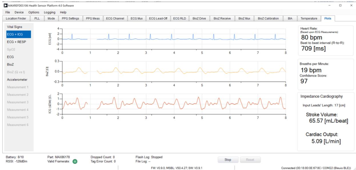
Figure 39. Example ICG Plot Tab
