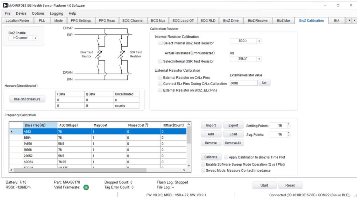
Figure 63. BioZ Calibration Tab
