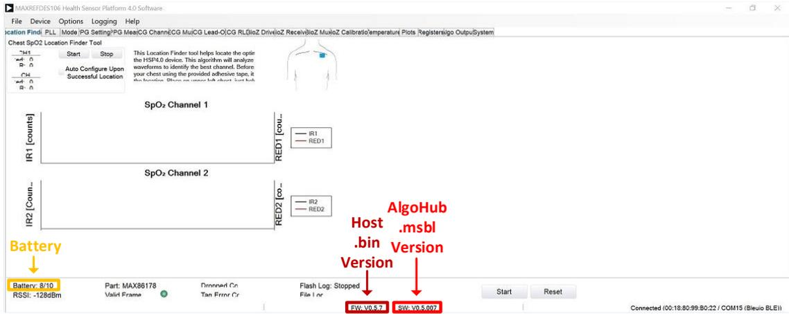
Figure 19. Battery Level, Host .bin Version, Algo Hub .msbl Version
