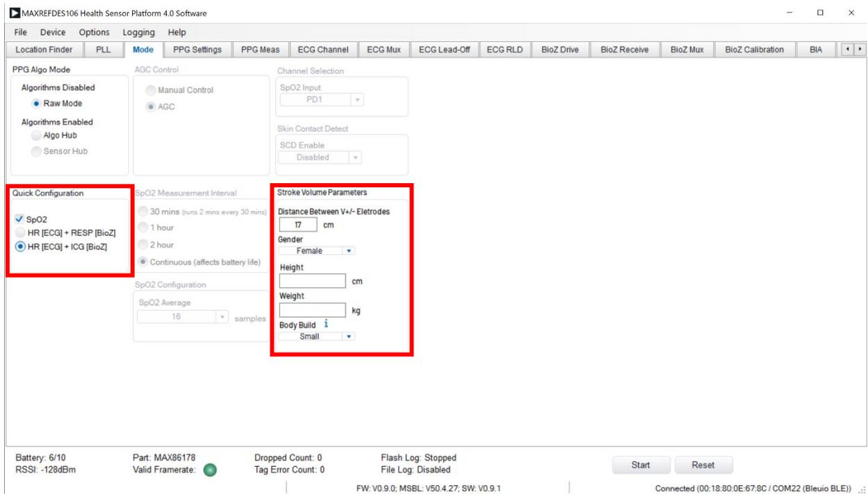
Figure 31. Mode Tab: Select HR [ECG] + ICG [BioZ] and Enter Stroke Volume Parameters
