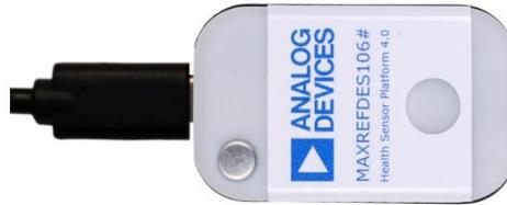
Figure 16. Connect USB-C Cable to the MAXREFDES106#
