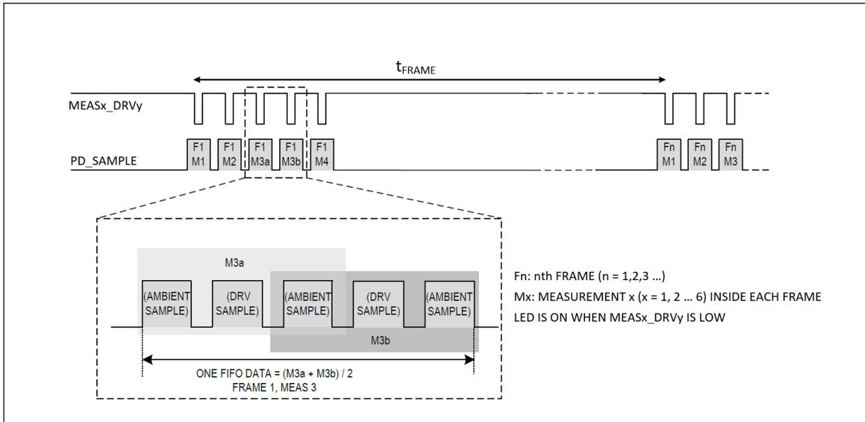
Figure 23. Frame with Measurement Averaging. MEAS3 has Two Sample Averaging, Before Being Pushed to FIFO as One Sample
