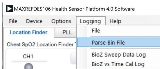
Figure 71. The Built-In Parser Processes, Converts, and Saves Flash Log Data to .csv Files
