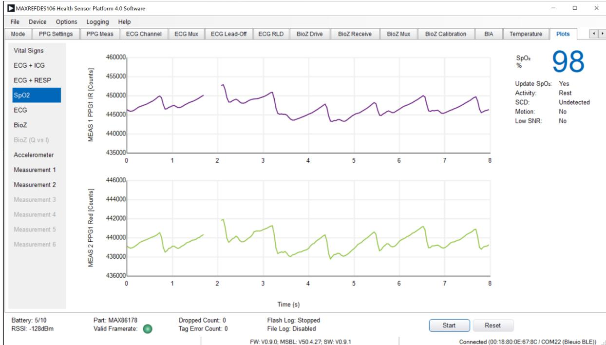
Figure 24. Example of Raw PPG Measurement Output
