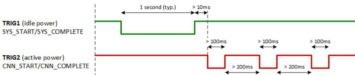
It is important to ensure the timing and sequence of the energy accumulation mode signals as described in the figure above.
