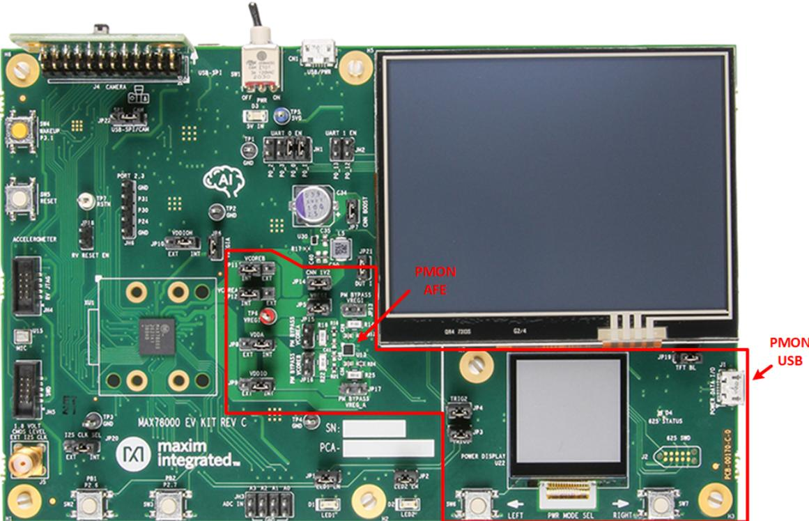
On the MAX78000EVKIT, JP3 and JP4 connect TRIG1 and TRIG2 signals from the MAX78000 to the PMON MCU to enable windowed power measurements.
