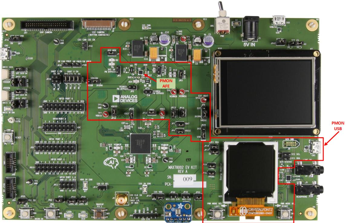
On the MAX78002EVKIT, JP18 and JP19 connect TRIG1 and TRIG2 signals from the MAX78002 to the PMON MCU to enable windowed power measurements.
