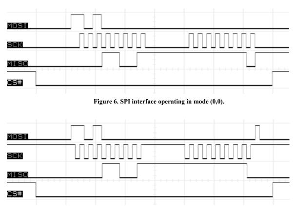
Figure 7. SPI interface operating in mode (1,1).
