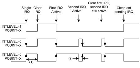
(1) Width determined by clearing the IRQ. (2) Fixed at ~20 usec.
