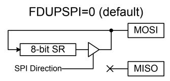
Figure 2. Half-duplex SPI interface.
