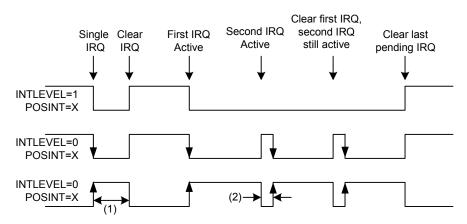
(1) Width determined by clearing the IRQ. (2) Fixed at ~20 usec.
