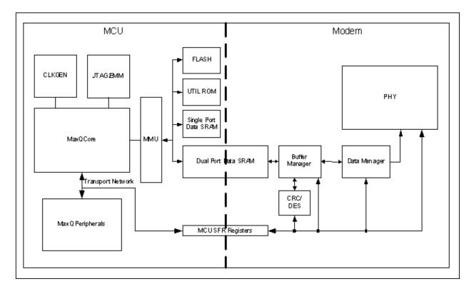
Figure1. MAX2990 Functional Diagram
