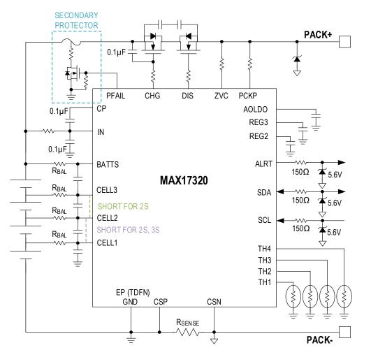
Figure 1. Example circuit schematic.
