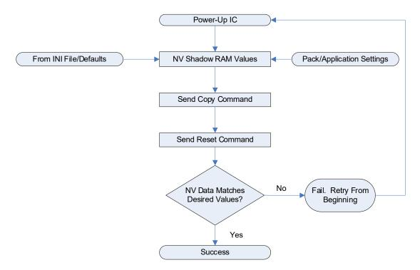
Figure 4. Nonvolatile memory loading process.
