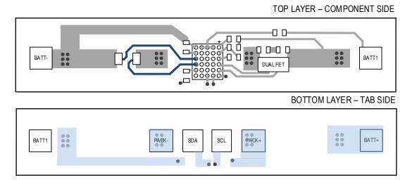
Figure 2. MAX17320 layout example (only top and bottom layer shown).
