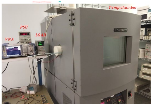
Figure 3.5.M. Block Diagram of How a Coupon Board is Used to Capture PoC S-Parameters under Varying Channels, Current Loads, and Temperatures
