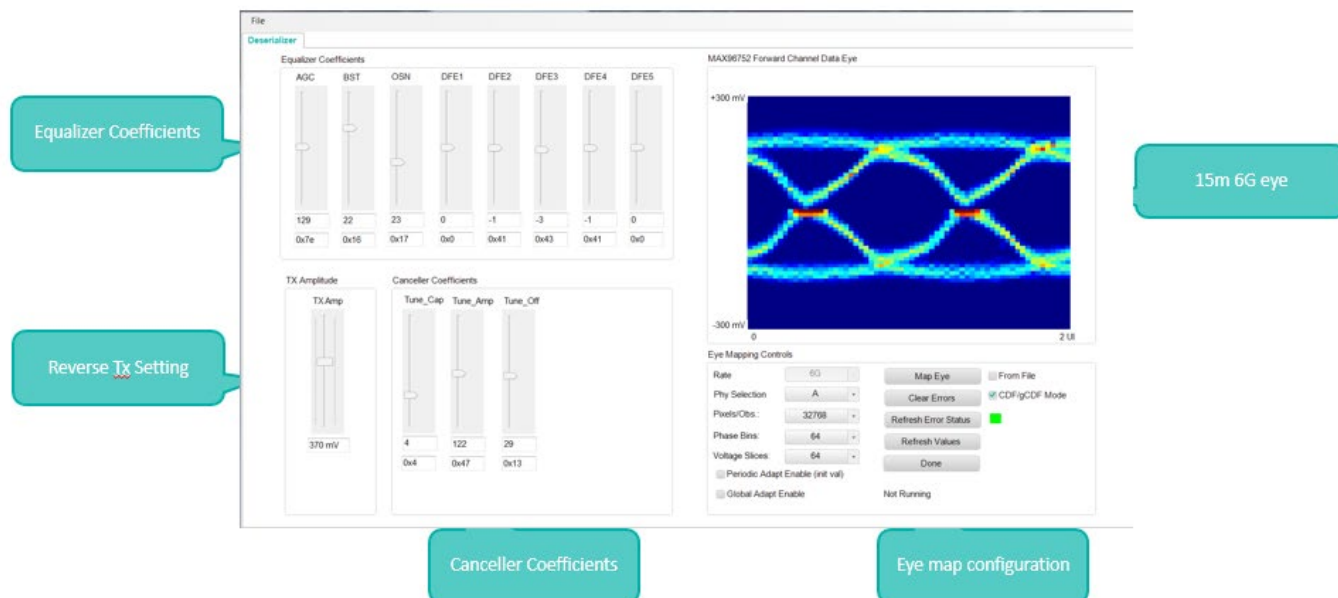
Figure 4.3.A: Eye Mapper Tool in GMSL GUI, 6Gbps Forward
