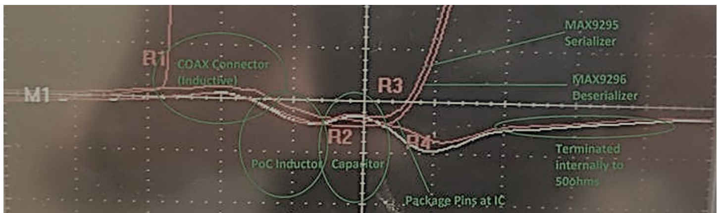
Figure 4.5.A: Example TDR of a PCB that Pass Channel Specifications. This is a Single-Ended Measurement (Coax System) with Rise Time = 100ps, x-axis scale = 200ps/div, y-axis scale = 5Ω/div Centered Around 50Ω
