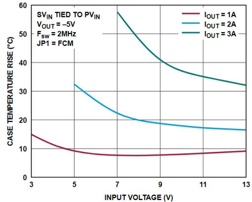
Figure 2. Case Temperature Rise vs.  $V_{IN}$
