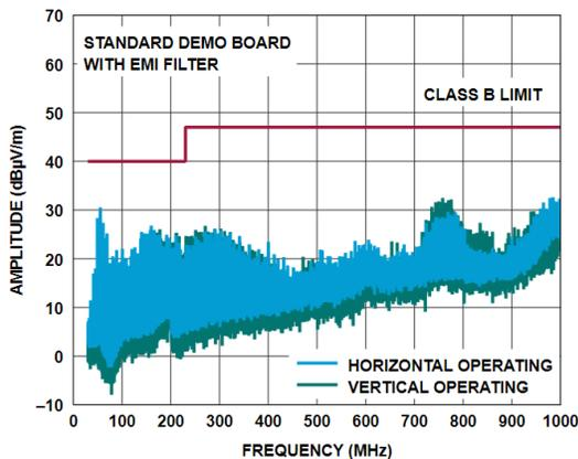
Figure 3. CISPR32 Radiated EMI Performance
