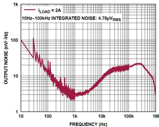
Figure 4. Noise Spectral Density
