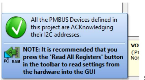
5. In the toolbar, click the **R** (RAM to PC) icon to read the RAM from the LT7170-1. This reads the configuration from the RAM of the LT7170-1 and loads it into the GUI.
