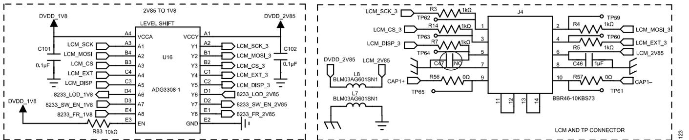
Figure 23. Level Shifter and Display Connections
