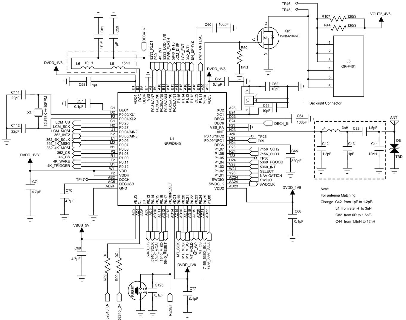
Figure 21. Microcontroller Connections
