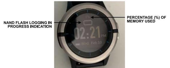
Figure 20. NAND Flash Logging Indicator with Percentage of Memory Used
