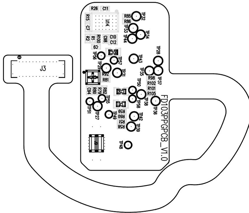
Figure 38. Optical PCB Layout Top View
