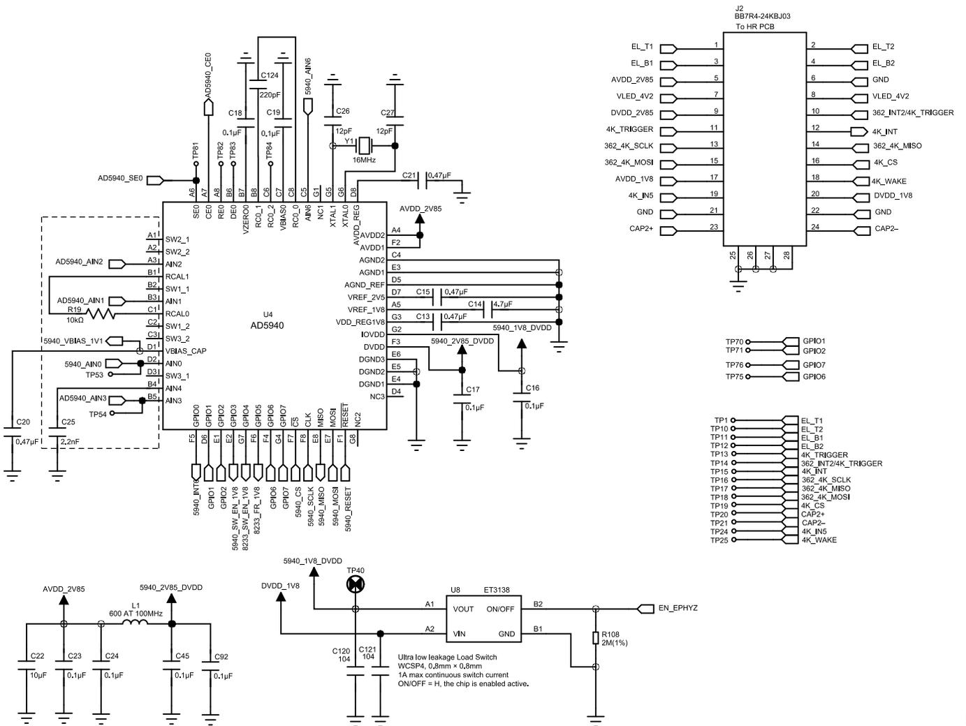
Figure 25. AD5940 Circuitry and Connection to Optical Board
