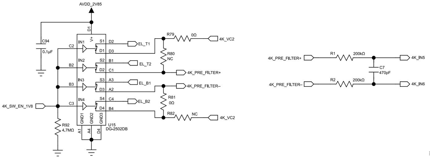
Figure 33. Electrode Connections for ADPD4100
