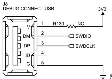
Figure 35. Debug Board Connector Pinout
