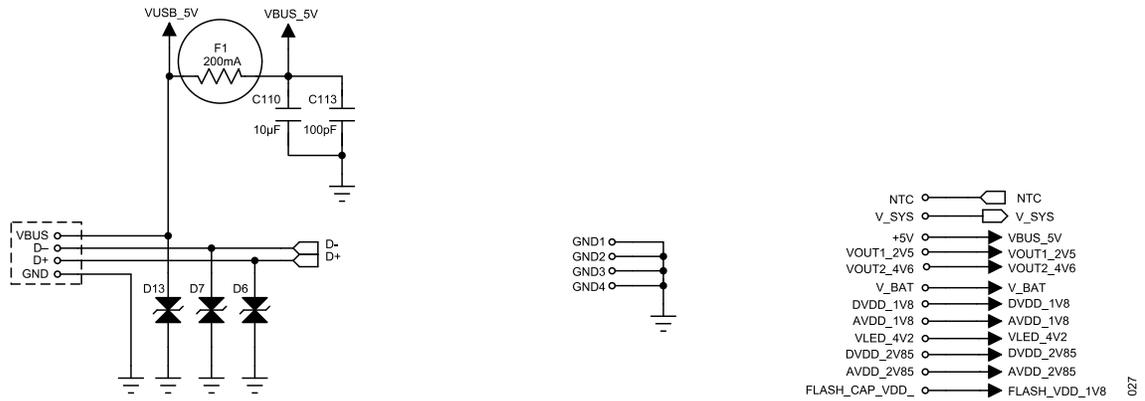
**Figure 27. USB Connection and Test Points**
