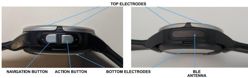
Figure 5. Connections and Buttons—Sides of Watch
