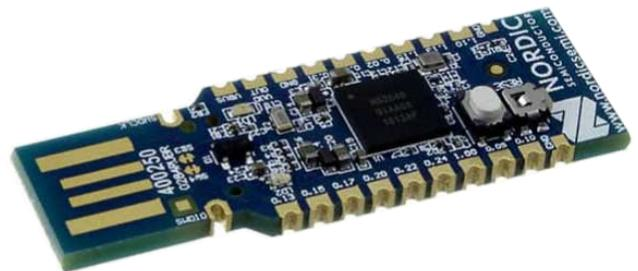
Figure 10. BLE USB PC Dongle (nRF52840)
