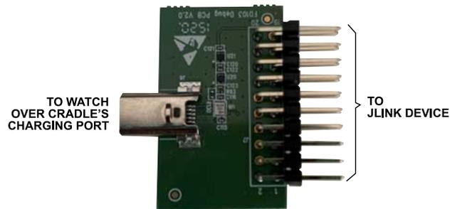
Figure 7. Firmware Debug Board
