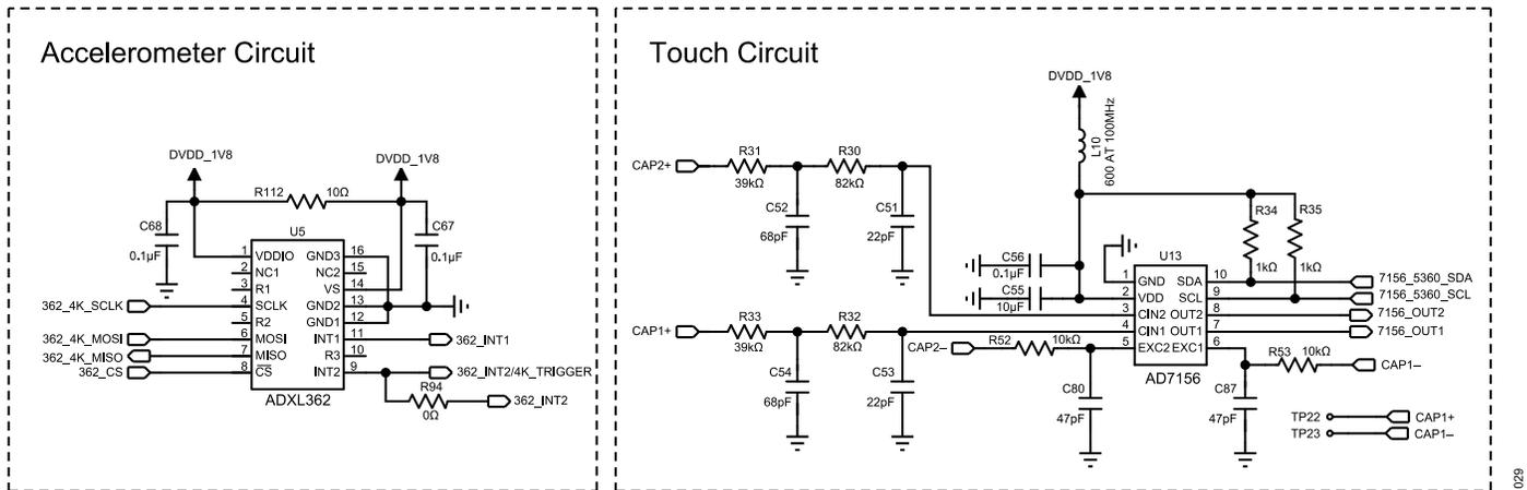
**Figure 29. Accelerometer and Capacitive Touch Circuits**
