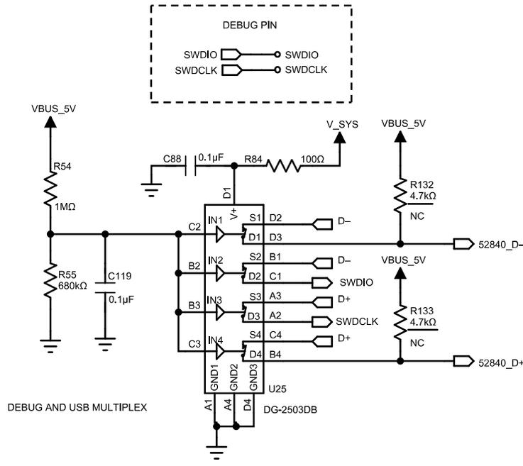
**Figure 30. Debug Switch (Communication and FW Programming)**
