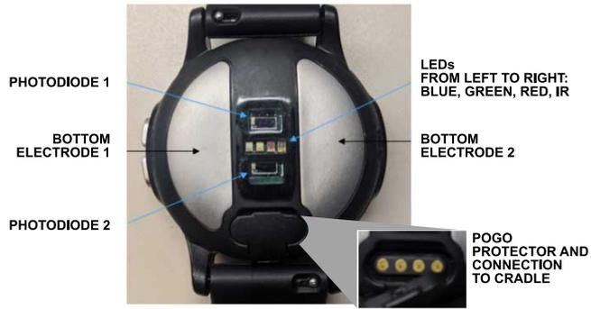
Figure 4. Connections and Buttons—Bottom of Watch
