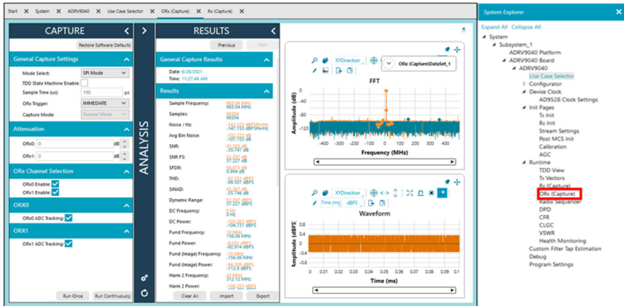
Figure 57. ORx0 and ORx1 Data Captured over JESD Link, with Tx LO + 10MHz Input Tone Applied to ORx0
