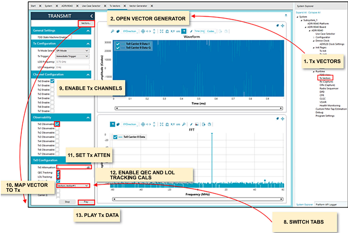
Figure 49. Tx Vectors Page is Used to Enable Tx Channels, Map Vectors to Each Enabled Tx, and Plot the Baseband Vectors
