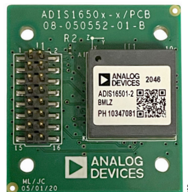
Figure 1. ADIS16501-2/PCBZ IMU Top View
