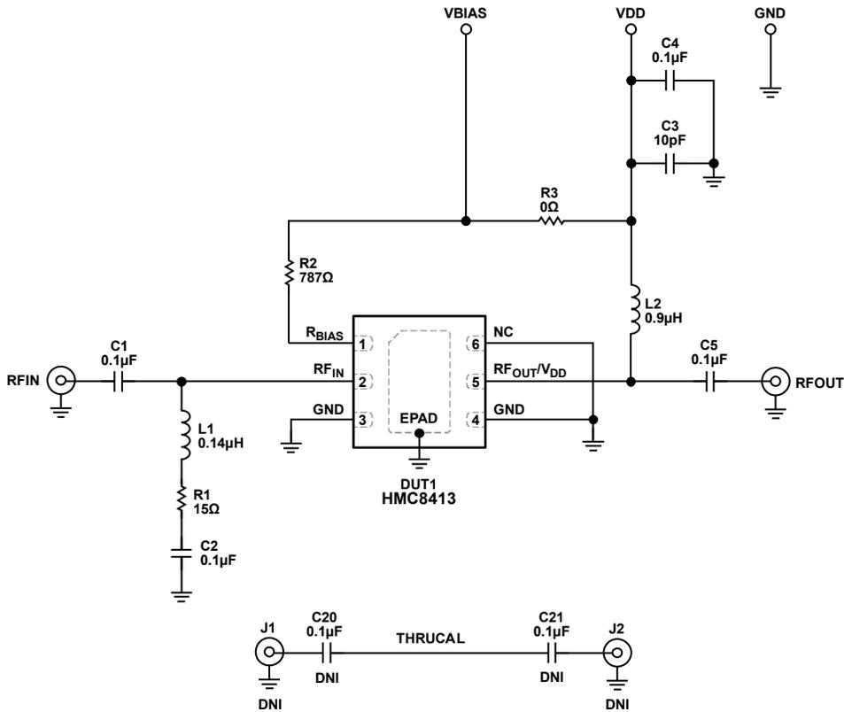
Figure 4. EV1HMC8413LP2F Schematic
