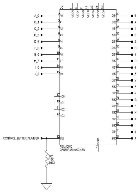
Figure 3-4: Example of a Bus Switch
