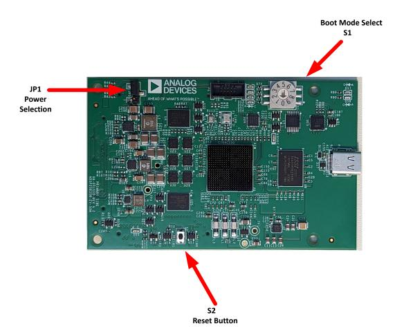
Figure 3-6: Switch/Jumper Locations
