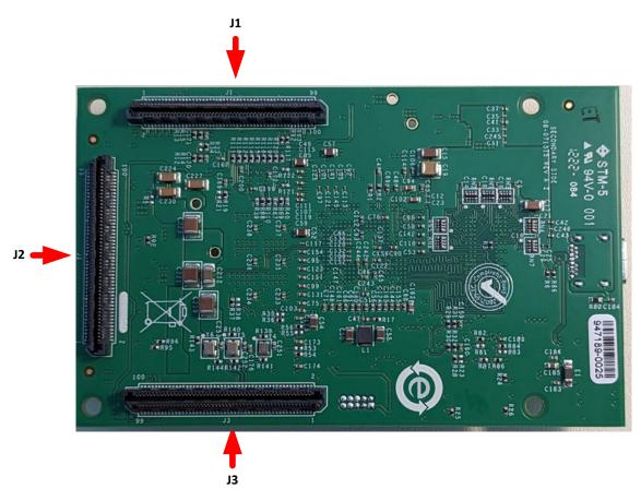
Figure 3-9: Connector Locations Bottom View
