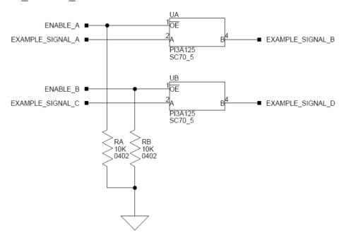
Figure 3-2: Example of Individual FET Switches
