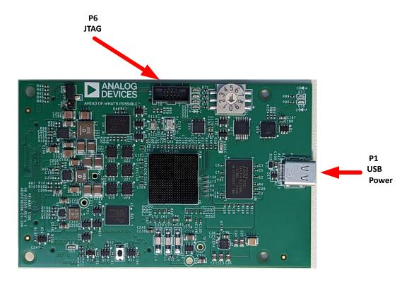
Figure 3-8: Connector Locations Top View
