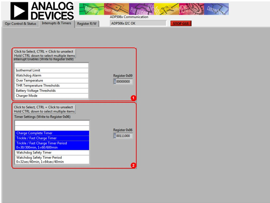
Figure 3. ADP5062 Evaluation and Design Software GUI, **Interrupts & Timers** Tab
