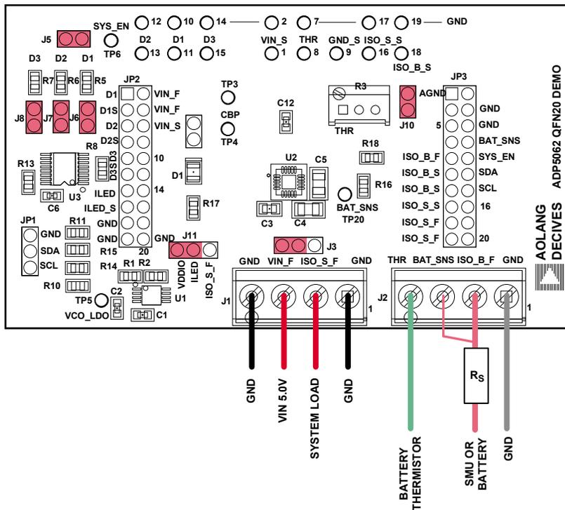
Figure 5. ADP5062CP-EVALZ Typical Operation Setup
