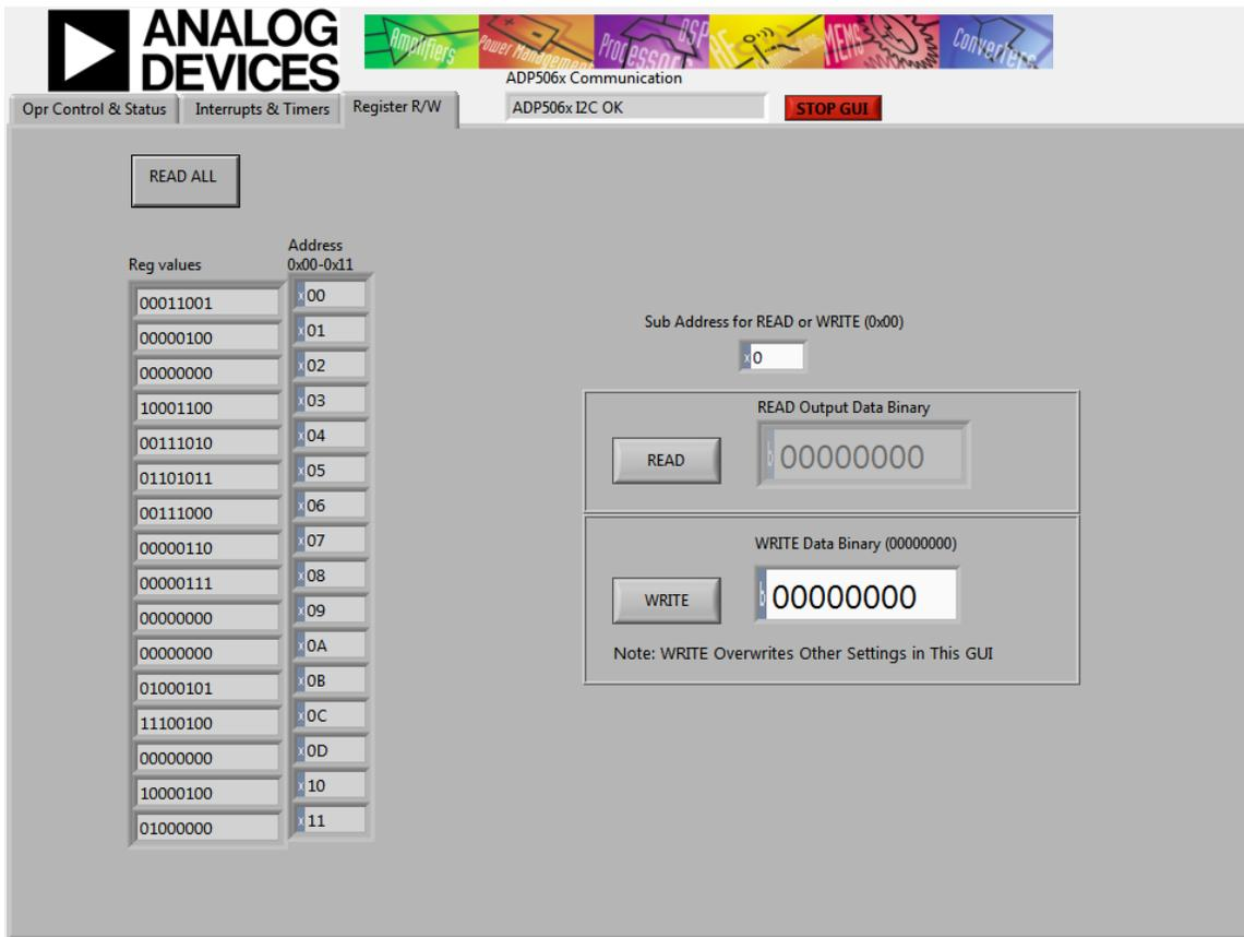
Figure 4. ADP5062 Evaluation and Design Software GUI, Register R/W Tab
