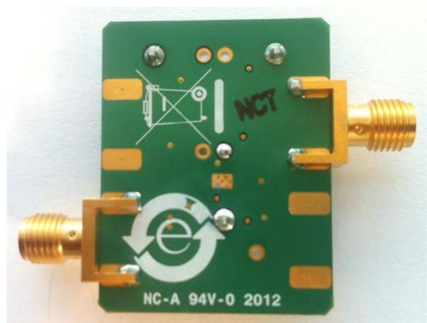
Figure 2. [ADA4432-1BCP-EBZ](#) Evaluation Board, Secondary Side
