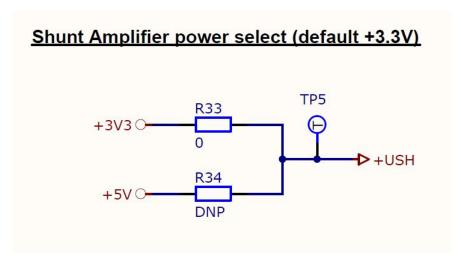
Figure 2: Power supply select for shunt amplifiers
