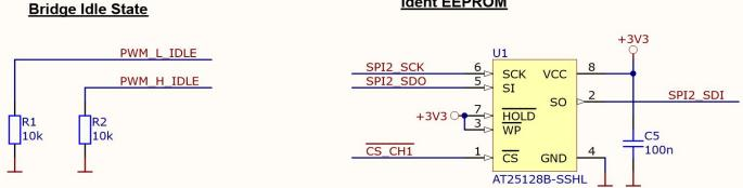
The evaluation board can be automatically recognized when Ident EEPROM is properly configured. This part is only needed on an Evaluation board for user convenience.
