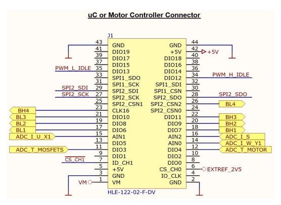
Figure 1: 44 pin Motor Controller Connector
