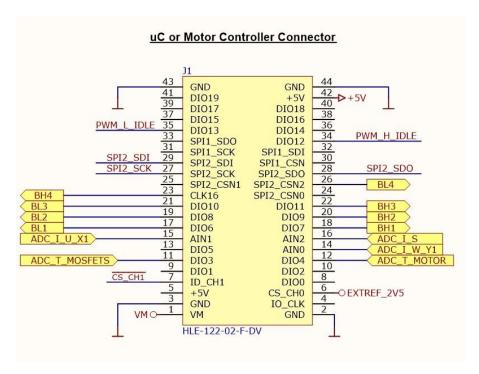
Figure 1: 44 pin Motor Controller Connector
