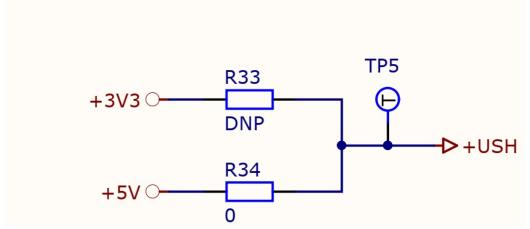
Figure 3: Power supply select for shunt amplifiers
