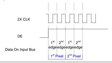
Table 8 YCbCr 4:2:2 (8 bits) DDR with Separate Syncs: Input ID = 6, right justified (R0x48[4:3] = '01')
