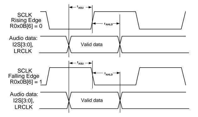
Figure 4 Timing for S/PDIF Audio Interface
