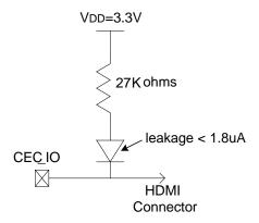
An example schematic is shown in <u>Figure 25</u>. For a complete set of reference schematics and PCB layout example, contact <u>ATV\_VideoTX\_apps@analog.com</u>.
