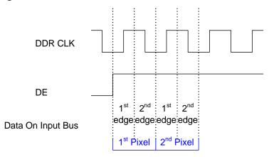
Figure 9 DDR DE timing - Register 0x16[1] = 0
