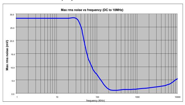
Figure 23 LC Filter Transfer Curve
