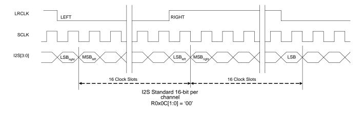
Figure 12 Serial Audio – Right-Justified
