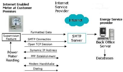
An Internet-enabled modem within a meter helps communicate the billing information periodically, enabling the service provider to not only generate timely bills, but also to understand energy demand patterns, failure and tamper identification. In addition, it enables the utility to offer energy at lower tariffs by adding the total demand of groups of companies or users.
