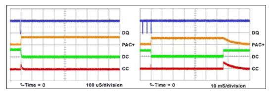
**Case K: Swap Command Sleep, Falling Edge of PS, PMOD = 1, SWEN = 1, DQ = 0, Cell > V<sub>UV</sub>** If the device has been swapped into Sleep Mode, SWEN is 1, PMOD is 1, DQ is low, and the cell voltage is above  $V_{UV}$ , then the device enter Active Mode 450µs after a falling edge on PS. The pins react the same as Case J for the first 2s. However, because PMOD is 1 and DQ is low, the device reenters Sleep Mode after 2s.
