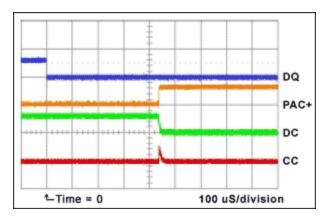
**Case L: Swap Command Sleep, Falling Edge of PS, PMOD = 1, SWEN = 1, DQ = 1, Cell > V**<sub>UV</sub> If the device has been swapped into Sleep Mode, SWEN is 1, PMOD is 1, DQ is high, and the cell voltage is above V<sub>UV</sub>, then the device enters Active Mode 450µs after a falling edge on PS. The pins react the same as Case J.
