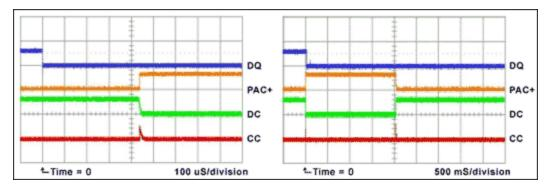
**Case M: Swap Command Sleep, Swap Command, SWEN = 1, DQ = 1, Cell > V**<sub>UV</sub> If the device has been swapped into Sleep Mode, SWEN is 1, and DQ is high, and the cell voltage is above V<sub>UV</sub>, then the device enters Active Mode on the next rising edge of DQ following a Swap Command to the Net Address of the device under test. Both CC and DC are driven low immediately, which enables PAC+.
