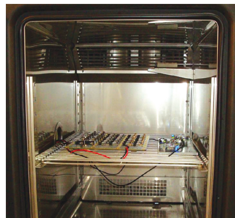
Figure 1. SmartMesh Nodes Operating in a Temperature Chamber
