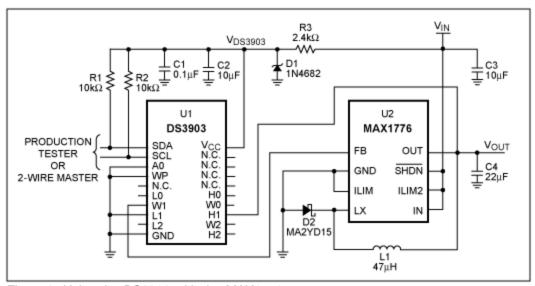
Figure 2. Using the DS3903 with the MAX1776.
