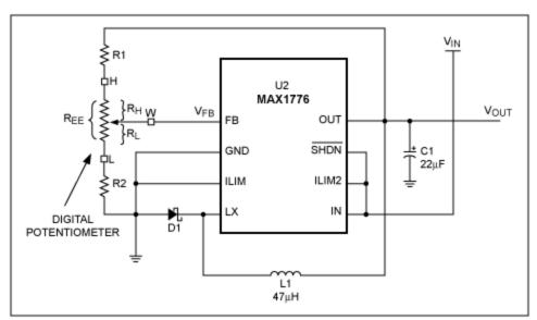
Figure 6. Improving the circuit's precision by adding external biasing resistors.
