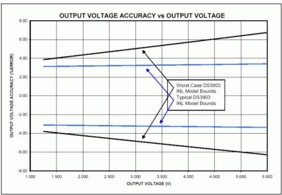
Figure 3. Output voltage accuracy as a function of desired output voltage.
