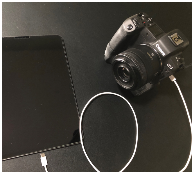
Figure 1. A digital camera connected to a tablet via a USB-C cable.
