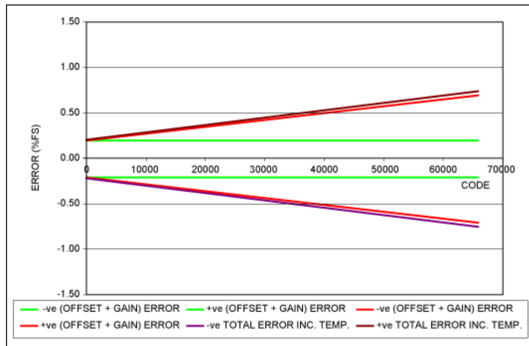
Figure 5. Example DAC output error vs. DAC code, V_{REF} = 2.5V .
