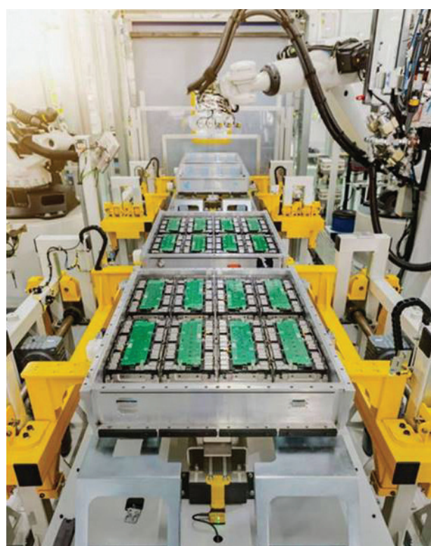
Figure 2. wBMS technology eliminates the signal wiring harness to enable automated, robotic production of complete battery packs.
