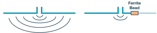
Figure 6. Use of ferrite bead to reduce effective dipole.
