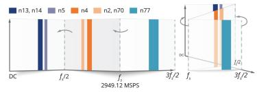
This illustrates spectrum folding back onto the first and second Nyquist zone creating aliases. Using a common sample rate, 2949.12, band n77 (C-Band) will alias with bands n2, n4, n5, n13, n14 and n70, increasing filter requirements, adding weight, and cost.
