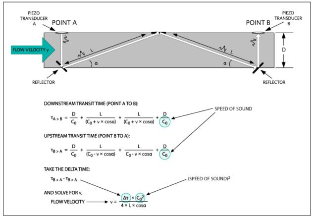
Figure 1. Example time-of-flight difference calculation.
