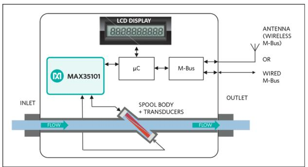
Figure 2. Water meter ultrasonic time-of-flight solution features the MAX35101 time-to-digital converter with analog front-end (AFE).
