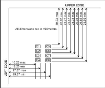
Figure 2. Contact dimensions and location.
