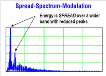
Figure 5b. Maxim's Spread-Spectrum-Modulation Mode.
