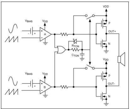
Figure 2. Mono Class D Amplifier Topology.
