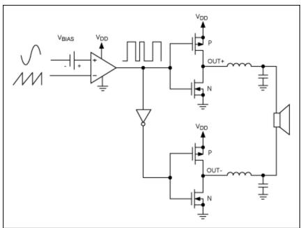
Figure 1. Conventional Pulse-Width-Modulation Topology.
