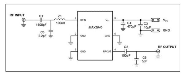
Figure 14. EV kit schematic for the MAX2640 at 315MHz.
