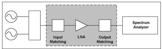
Figure 16. Measurement setup for LNA gain and IIP3.
