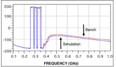
Figure 6. S22 (phase) comparison between simulation and bench measurement.
