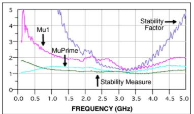
Figure 11. Stability measurement, stability factor, source stability factor, and load stability factor for the second test case.
