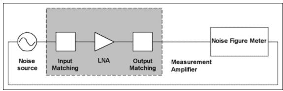
Figure 17. Measurement setup for noise figure.
