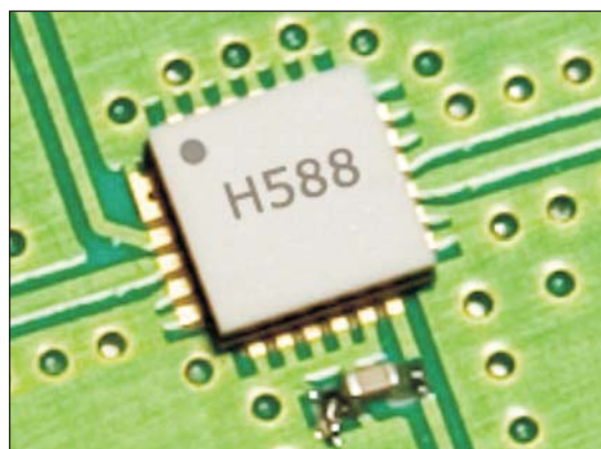
Figure 1 • Photograph of the HMC588LC4B Wideband VCO in a 4 × 4 mm SMT package, mounted to a PC board.
