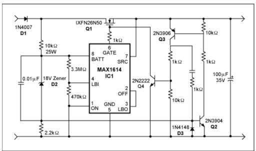
Figure 1. This circuit protects a load (connected to the right pair of terminals) against undervoltage and
