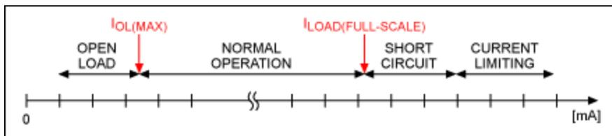
Figure 2. Operation ranges for the current-sense amplifiers.
