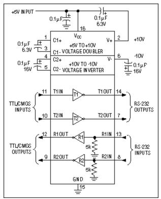
Figure 2. The MAX202E works off a single 5V power supply;  $\pm 10V$  is generated using on-board charge pumps and four external capacitors.
