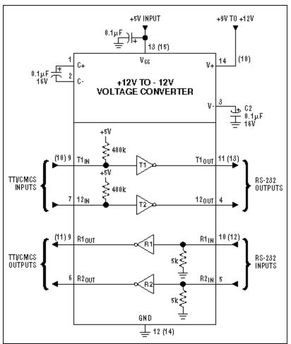
Figure 7. The MAX201 is an example of a part that is powered from a 5V and 12V supply. The -12V is generated using an on-board charge pump and two external capacitors.
