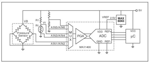
Figure 1. Circuit directly measures the variables needed to calculate the actual pressure (excitation voltage, temperature, and bridge output).
