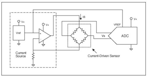
Figure 4. This circuit uses a current driven sensor powered by a conventional current source.
