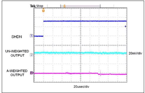
Figure 2. Data show the transient events associated with a low-offset, DC-coupled headphone amplifier
