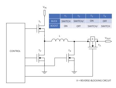
Figure 4. Buck-Boost Power Train Architecture and Operation Table
