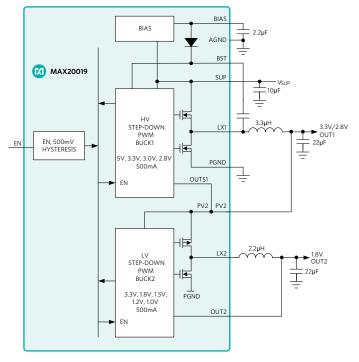
Figure 9. Dual Buck Converter Cascade
