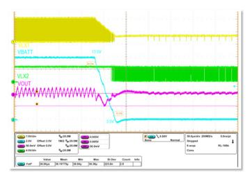
Figure 6. Negative Line-Transient Response
