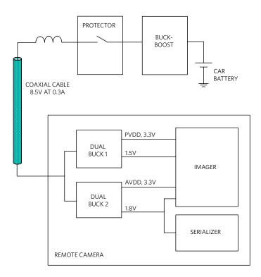
Figure 3. Remote Camera Single-Channel Detail
