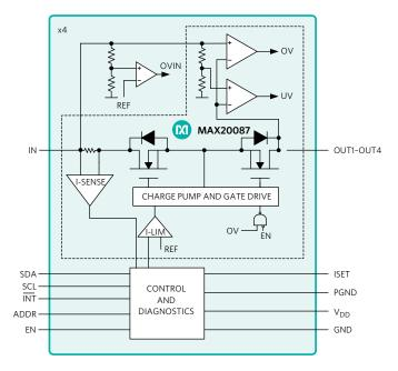
Figure 8. Input Current and Voltage Protection
