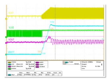
Figure 5. Positive Line-Transient Response
