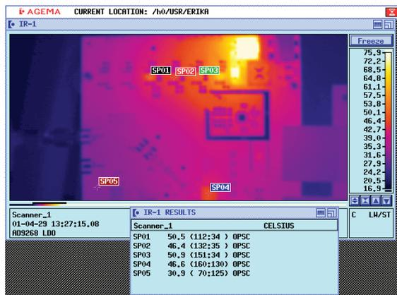
Figure 8. Thermal image of AD9268 evaluation board with linear power supply.
