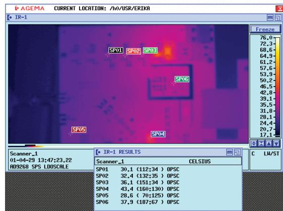
Figure 9. Thermal image of AD9268 evaluation board with ADP2114 supply.
