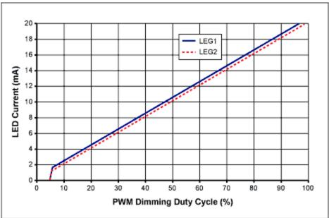
Figure 2. PWM dimming adjusts LED current and controls 1μA shutdown mode. Leg-to-leg current matching is good (better than 5%).
