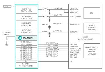
Figure 4. Fully Integrated AP Power Management
