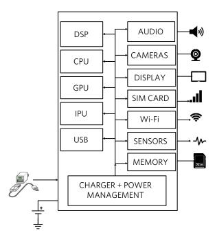
Figure 2. VR Headset Block Diagram
