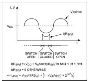
Figure 4. Switching-mode amplifier waveform.
