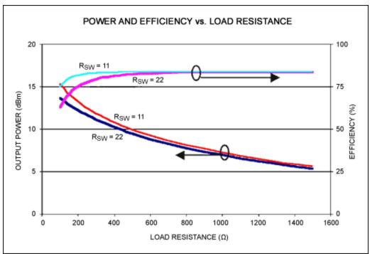
Figure 6. Ideal switching-mode amplifier performance vs. load resistance.
