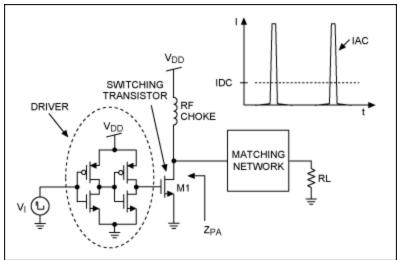
Figure 2. Schematic of a switching-mode amplifier.
