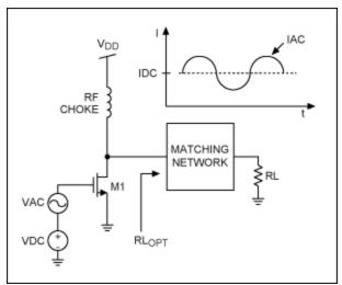
Figure 1. Schematic diagram of a class A amplifier.
