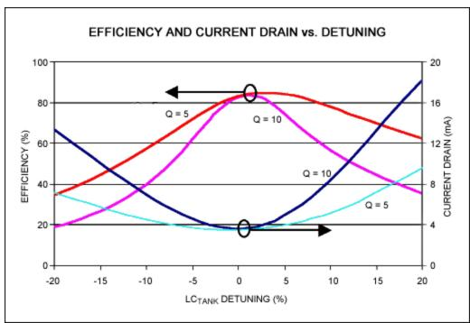
Figure 7. Ideal switching-mode amplifier performance vs. detuning.
