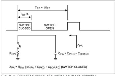
Figure 3. Simplified model of a switching-mode amplifier.
