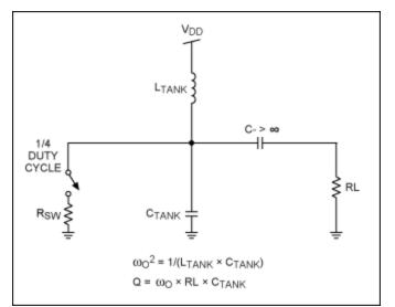
Figure 5. Simulation schematic for an ideal switching-mode amplifier.
